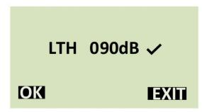
Set the desired level and enabled the alarm by using the arrow buttons. A tick denotes that the alarm is active; a cross denotes that the alarm is disabled. When set, press (a) to confirm.
